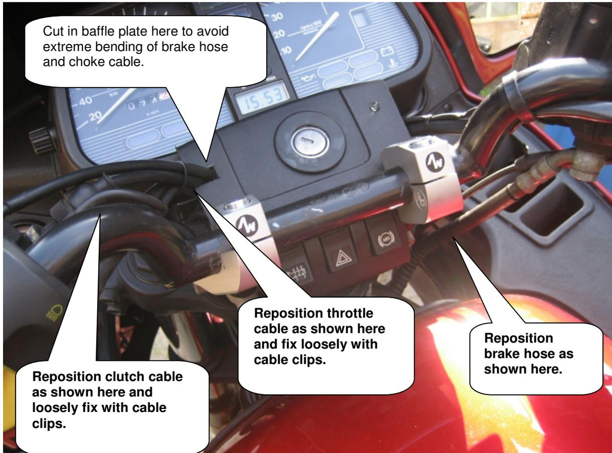
Finally fix all cables with cable clips and make sure that all cable and lines have enough play to avoid rubbing when the handlebar is completely turned.
