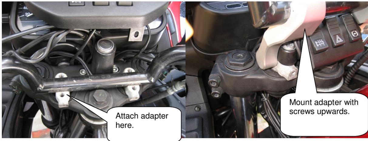
Hang out the clutch and throttle cable and put it aside so that both can be repositioned later. Fit the brake hose extension – as shown in the picture. Now the handlebar can be dismantled in order to fit both enclosed handlebar adapters.
